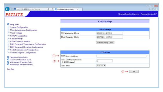
Fig. 4.3.2–1 Clock Setup screen for an NTP Server
