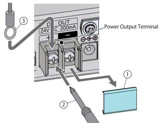
Fig. 2.4.2–1 Power Output Terminal
