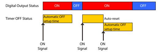
Fig. 3.1.5–1 Automatic Digital Output OFF Function detailed drawing
