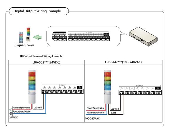
Fig. 3.1.1–2 Digital Output Wiring Example
