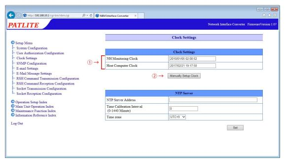
Fig. 4.3.1–1 Setup Screen before "Manually Setup Clock" button is clicked
