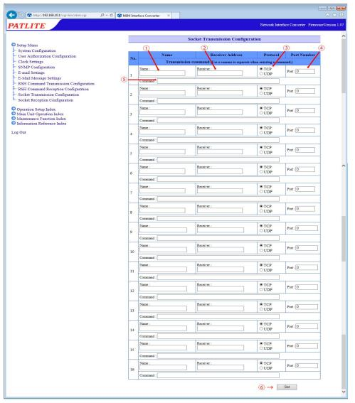
Fig. 4.9.0–1 Socket Transmission Configuration screen
