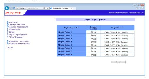
Fig. 4.20.0–1 Digital output operation setting screen
