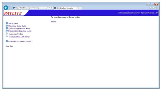
Fig. 4.22.0–2 Firmware Update Failure screen
