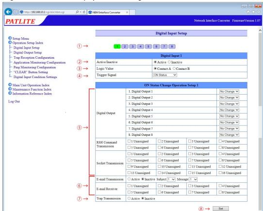
Fig. 4.11.0–1 Digital Input Setup Screen (when "ON Status" is selected)
