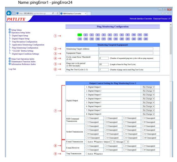
Fig. 4.15.0-1 Ping Monitoring Configuration Screen No. 1
