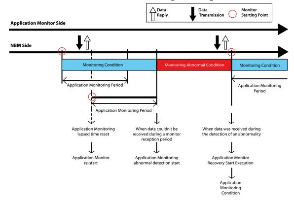
Fig. 3.10.0–1 Detail drawing of application monitoring operation example
