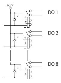
Fig. 3.1.6–1 Digital Output Circuit Schematic
