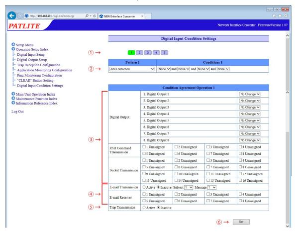
Fig. 4.17.0–1 Digital Input Condition Settings screen ("AND detection" pattern)
