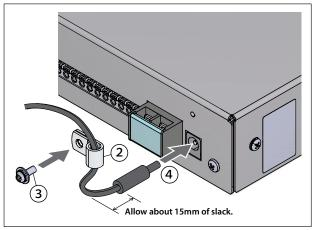
Fig. 2.5.0–2 Power Supply Switching Method
