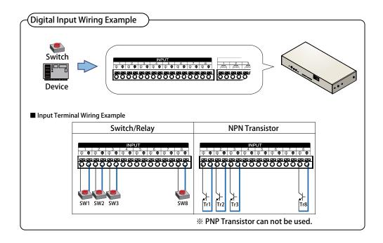
Fig. 3.1.1–1 Digital Input Wiring Example
