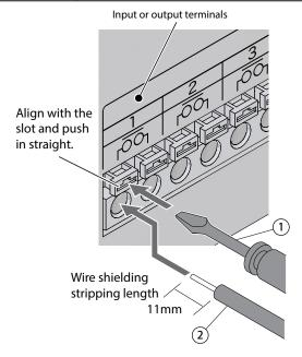
Fig. 2.4.1–1 Input/Output Wires
