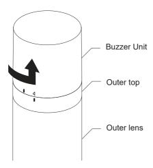
While holding the outer top or outer lens, turn the buzzer unit counter-clockwise to unlock it and lift it upward.
