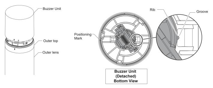
The rib inside of the Buzzer Unit fits into the groove when the Buzzer Unit has been removed from the product.
