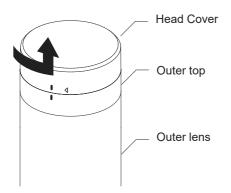
While holding the outer top or outer lens, turn the head cover counter-clockwise to unlock it and lift it upward.
